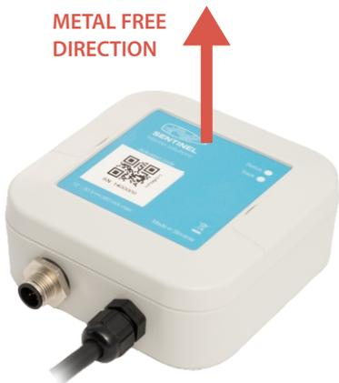
Sentinel Boat Monitor has internal GNSS and GSM antennas. The device should be mounted with the label facing upward to ensure optimal GNSS satellite reception (fig. 1). The sky view should not be obstructed with any metal objects. If metal above the device cannot be avoided, at least  $\frac{3}{4}$  of metal free area must be assured.
